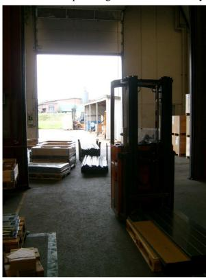
The picture shows that the articles en truck(s) form obstacle. Because of this the warehouse employee could not transport the finished boxes to the shipment dock. This results in finished boxes in the packaging area. This limits the space in the packaging area (see picture below).
