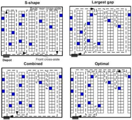
Figure 3.1 Routing heuristics for order picking
